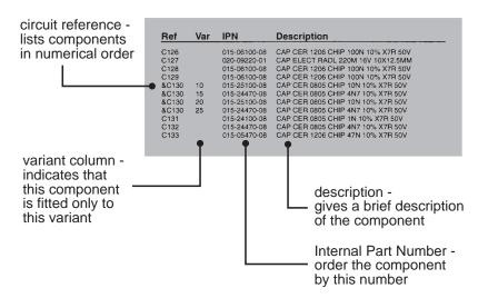
The miscellaneous and mechanical section lists the variant and common parts in IPN order.
